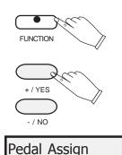
1. Press the FUNCTION button. The Function LED indicator will turn on. The first menu item is Touch which appears on the LCD display.
